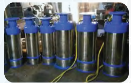
DEEP WELL PUMP UNIT
